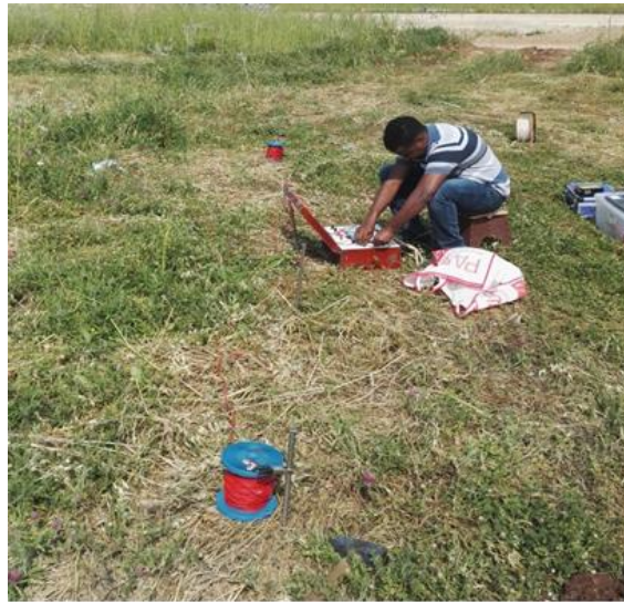
Figure 3. Obtaining data by applying the VES method in the study area
