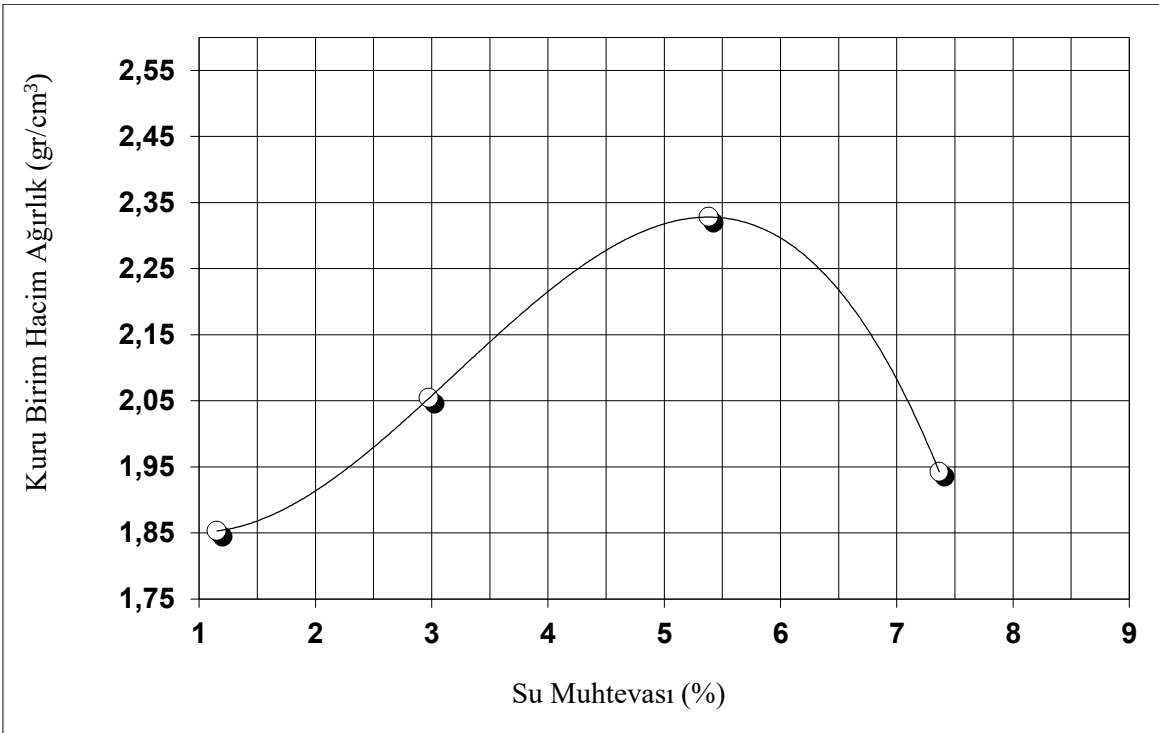
Figure 9. Unit volume weight-optimum water content graph of Viranşehir sample
