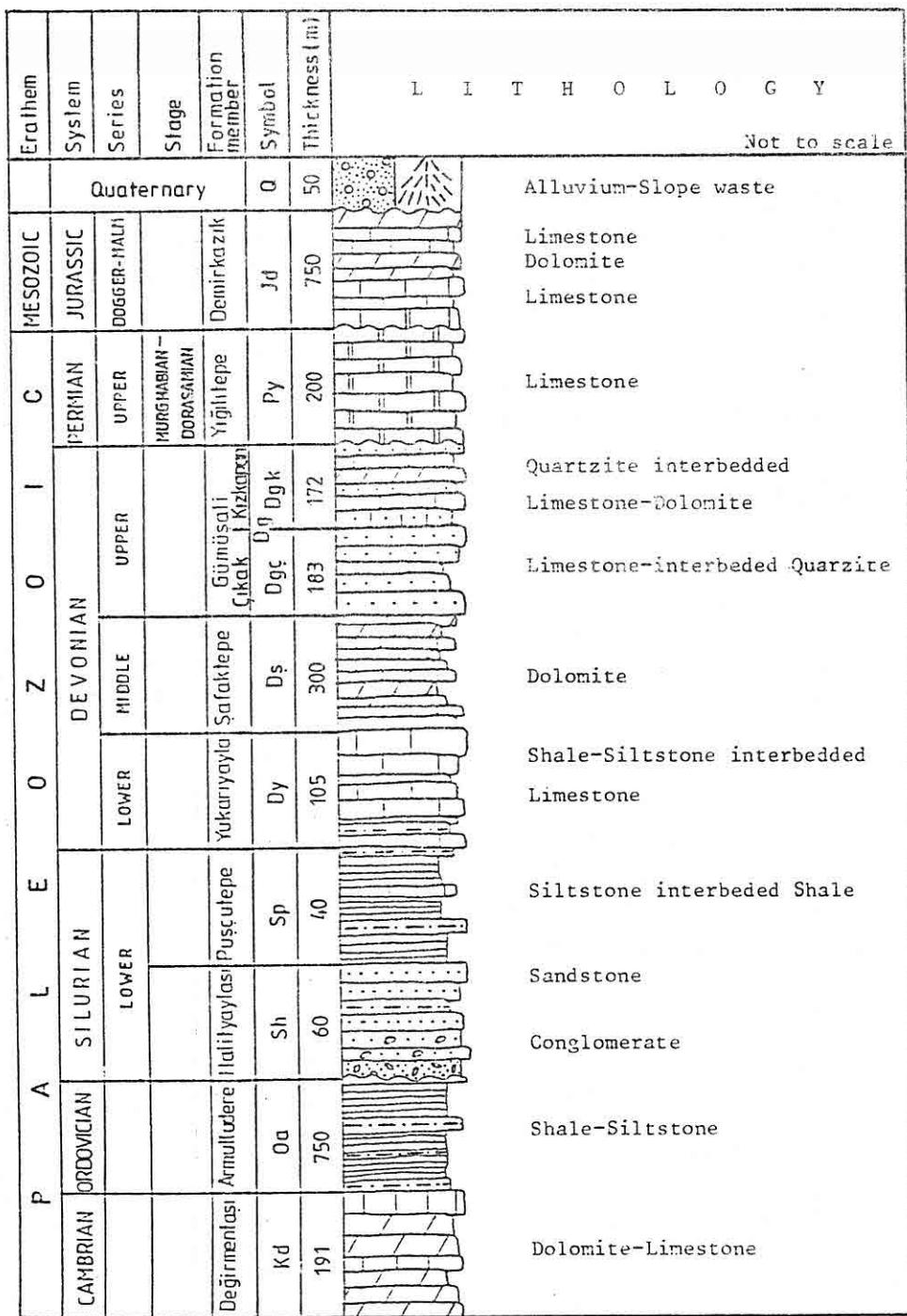
Figure 2. Generalized stratigraphic section of the Feke-Fekedağ (Adana) area.
