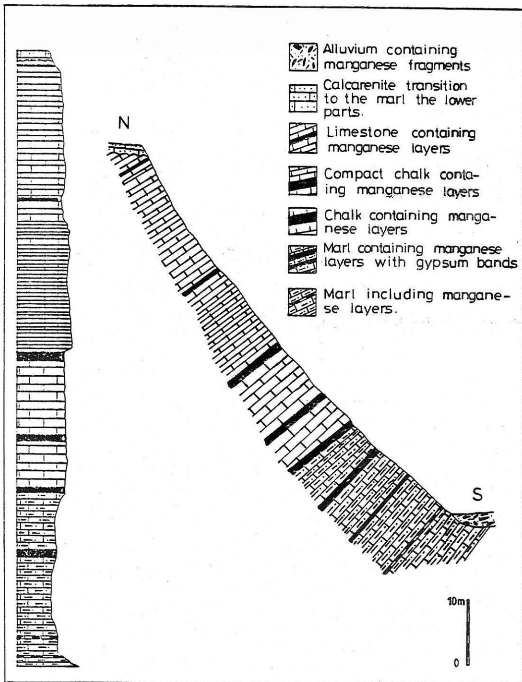
Figure 11. The vertical and horizontal sections of sedimentary manganese occurrences as nine levels south of Ziyamet (from Necdet) (25).
