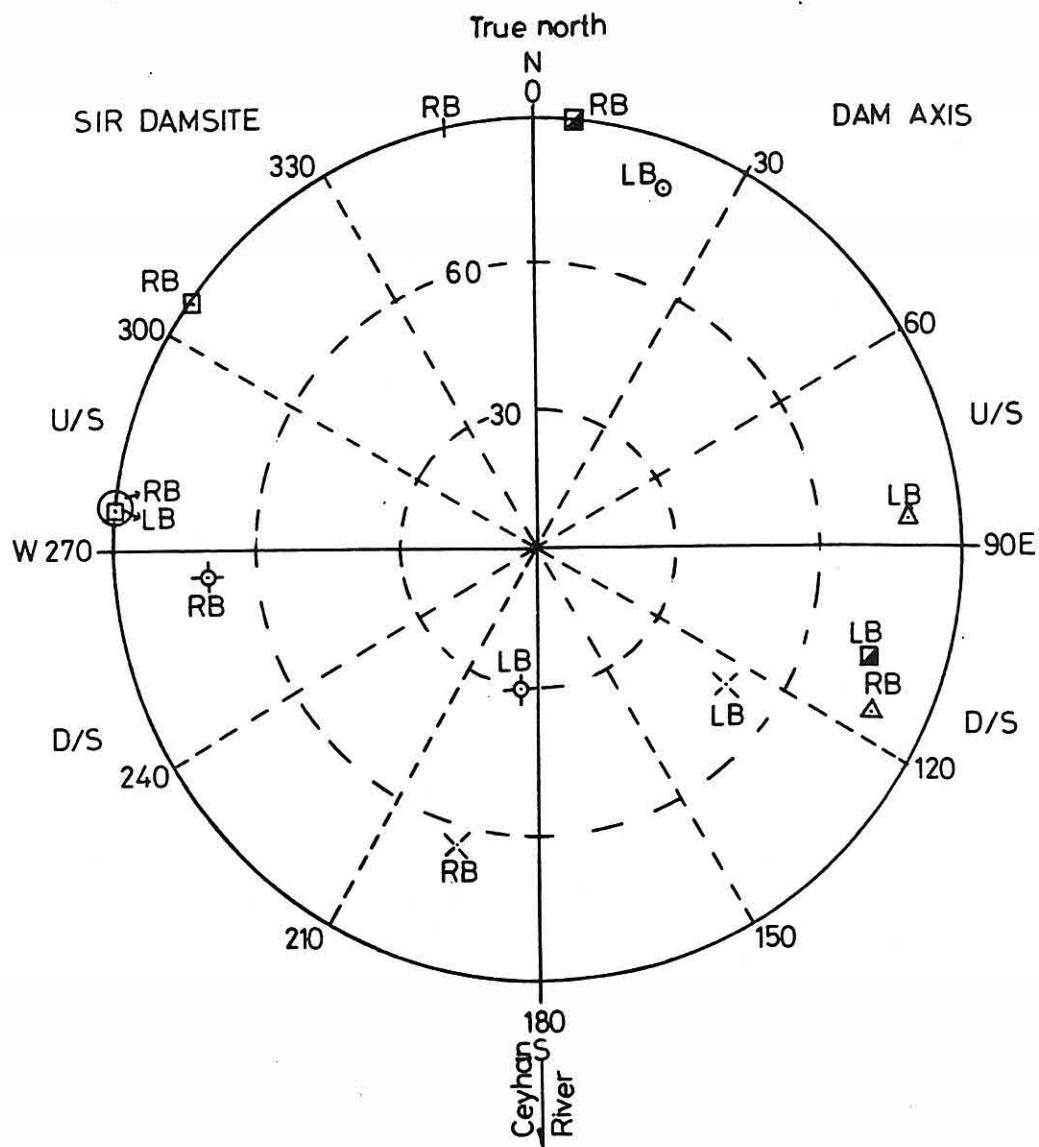
Figure 3. THE POLES OF THE JOINT SETS IN SIR QUARTZITE
