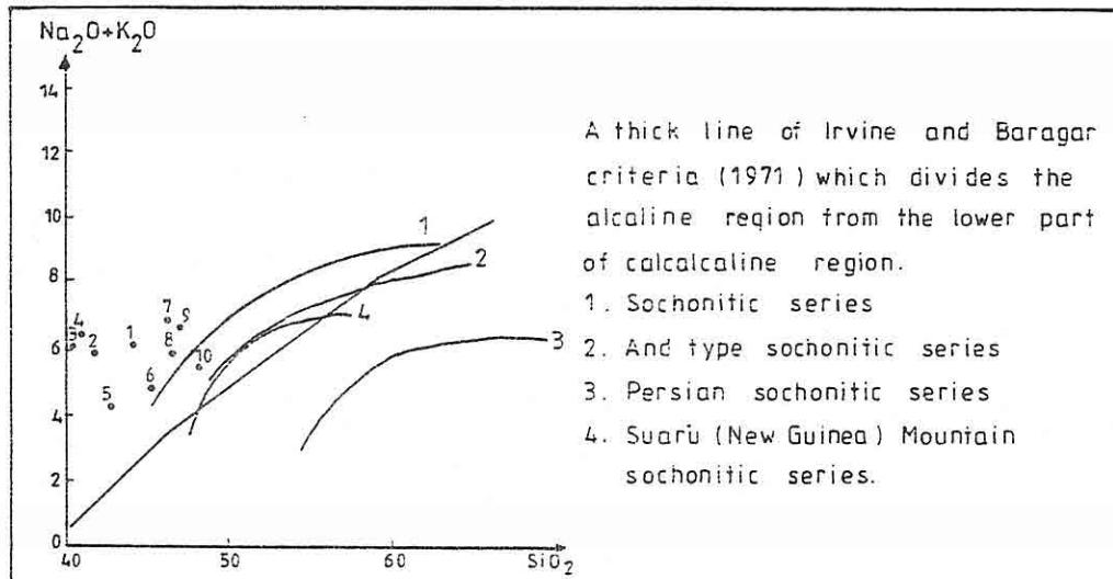
Figure 6. The distribution of Paleocene volcanics in alkaline diagramme (the points of 5-10 were taken from Baroz) (10).
